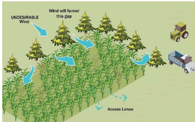
Figure 40 Undesirable gap effect of windbreaks
